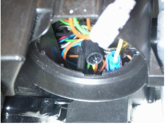
Next, connect the OEM connector to the LUX H8 connector as shown. Connect it with the inside tabs lining up.
