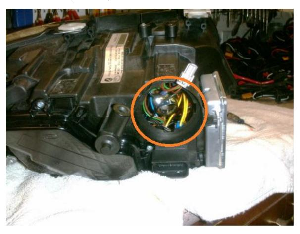
Inside the back opening, look for the small tab and press on it with your finger or the screw driver.
